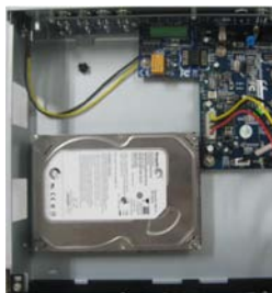
Fig 2.1 Connect HDD
